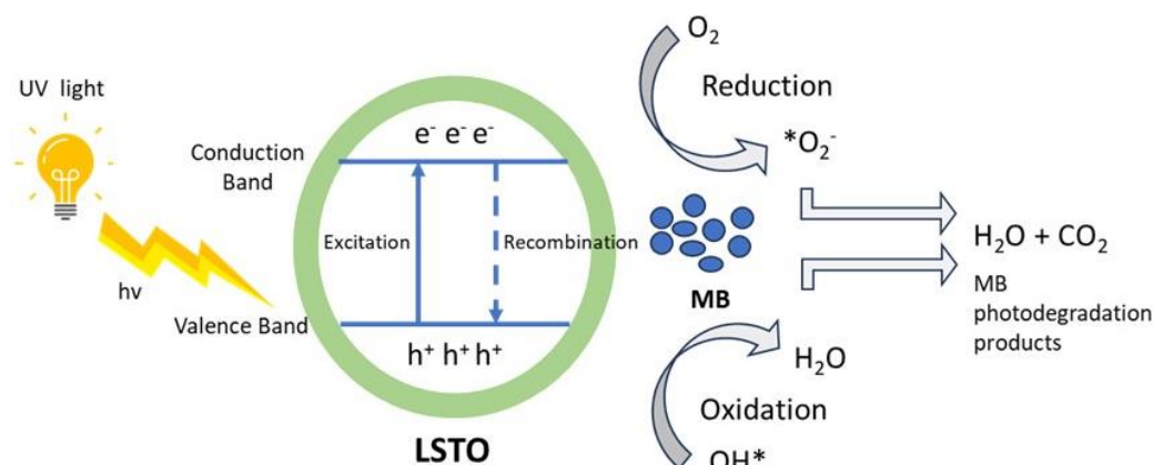
Fig. 6. Fundamental process of methylene blue photodegradation by LSTO samples
