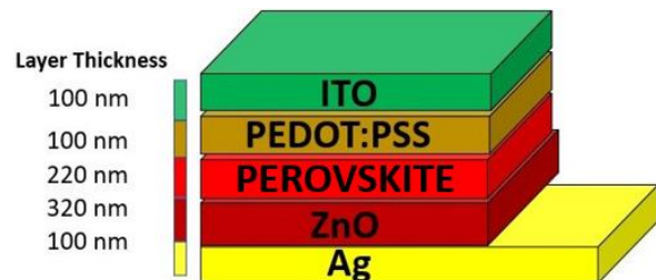
Fig. 16. Simulated Perovskite Solar cell with layer Thickness
