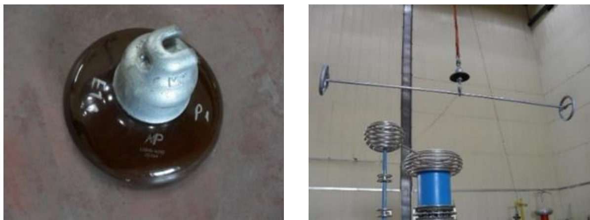
Fig. 16. The breakdown voltage experiment is according to the international standard of IEC-60383-01.
