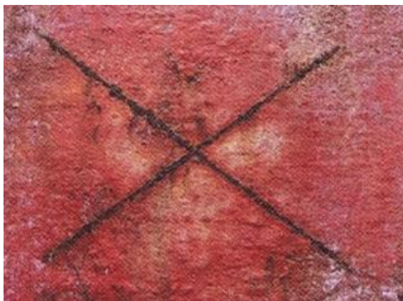
Fig. 15. The coated sample after 150 hours of emplacement under the salty-fog conditions according to ASTM-B117.
