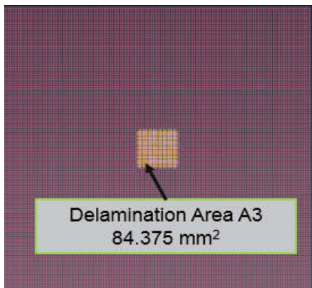
Fig. 3. Top view of delamination incorporated.
