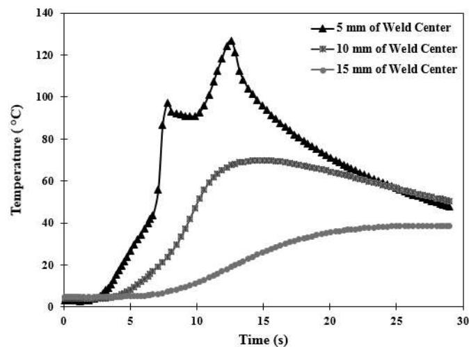
**Fig. 7.** Simulated top surface temperature distribution (1400 rpm–20 mm/min).
