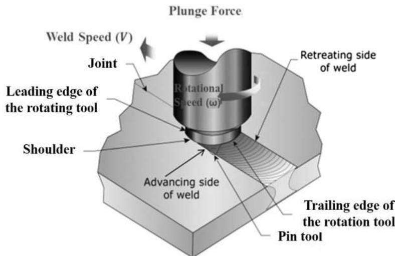
Fig. 1. Schematic of friction stir welding (FSW) process.
