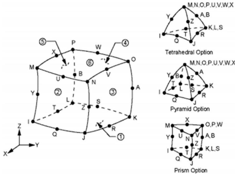
**Fig. 3.** Three dimensional thermal solid element SOLID226 [36].
