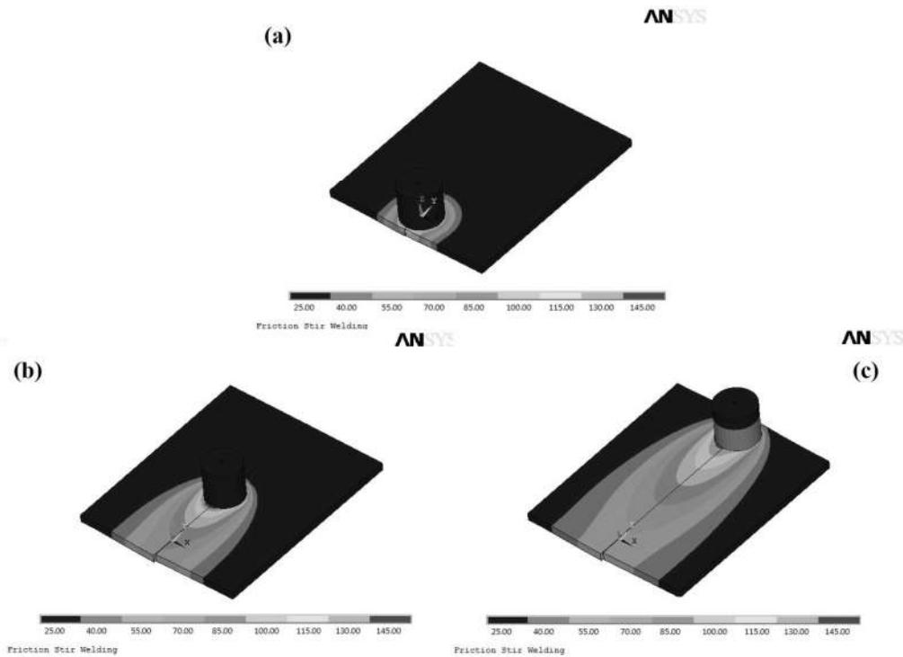
**Fig. 6.** Temperature map distribution at the (a) first, (b) second and (c) third load steps of the simulation (1400 rpm–20 mm/min).
