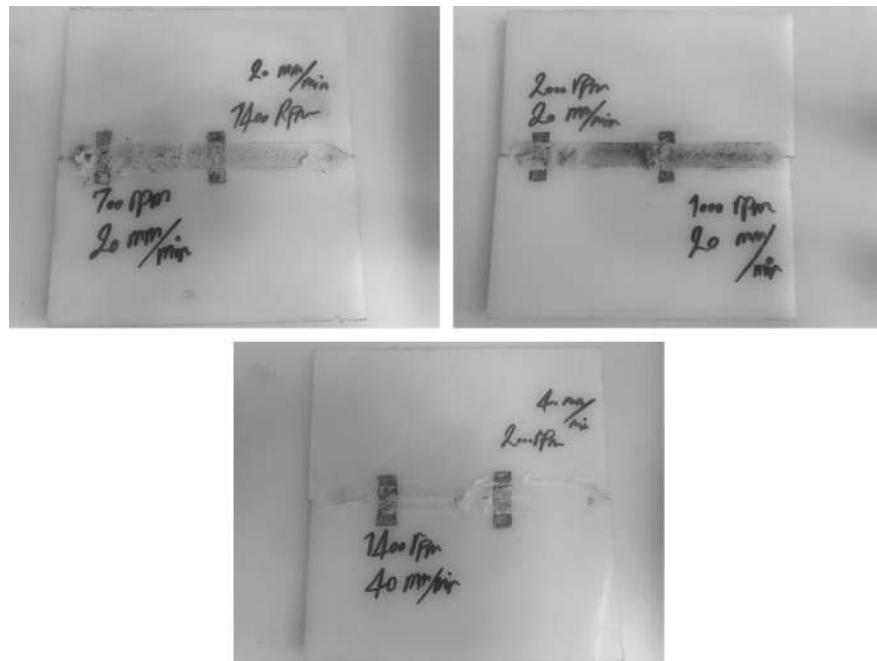
**Fig. 4.** Surface appearance of friction stir weld joints.
