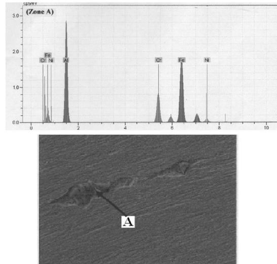
**Fig. 15.** EDX analysis combination A Area of spring steel 1.4568 microstructure after heat treatment (at 480°C , 80 min and cooling in air, then heating in oil bath 230°C for 60 min and cooling in cold water)
