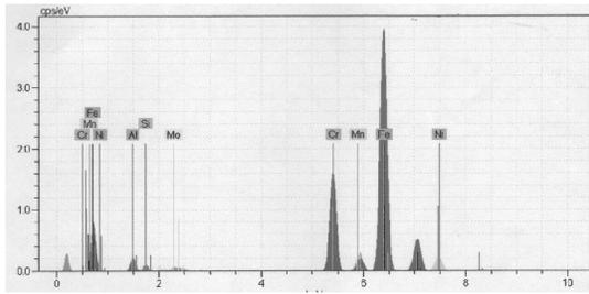
**Fig. 13.** EDX analysis of the spring steel 1.4568 microstructure after heat treatment (at 480°C for 80 min and cooling in air, then heating inside oil bath 230°C for 60 min and cooling to cold water).
