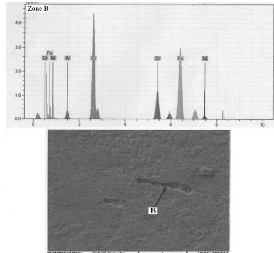
**Fig. 16.** EDX analysis composition B Area of spring steel 1.4568 microstructure after heat treatment (at 480°C , 80 min and cooling in air, then heating in oil bath 230°C for 60 min and cooling in cold water).
