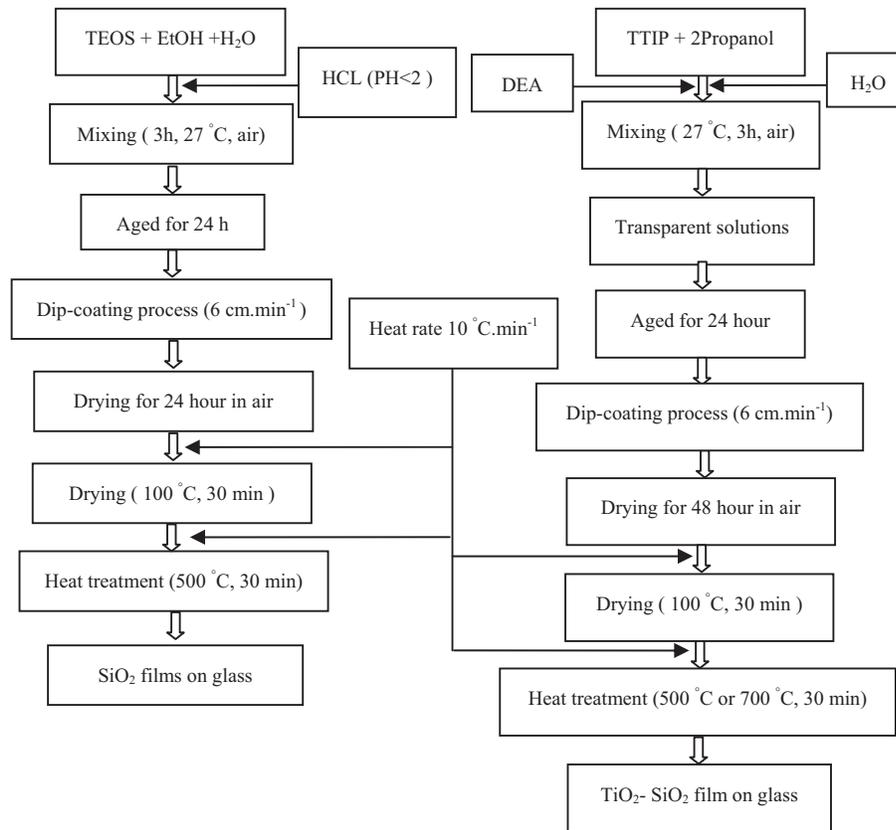
Fig. 1. Experimental procedure used in this research (left: preparation process of SiO<sub>2</sub> films, right: the preparation process of TiO<sub>2</sub>-SiO<sub>2</sub> films).
