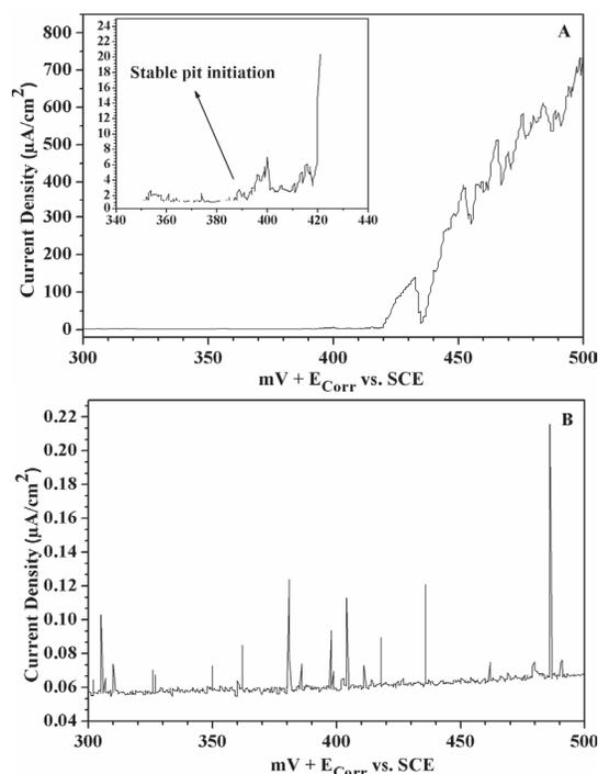
**Fig. 3.** Slow ramp anodic polarization of (A) as-received (inserted micrograph shows potential which is pitting corrosion started) and (B) electropolished 316 StSt with 3mV/min scanning rate in potential range of 300-500 mV higher than  $E_{corr}$
