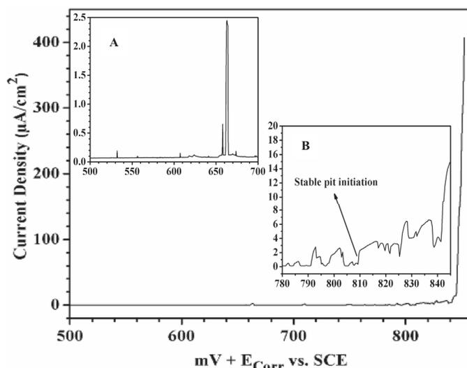
Fig. 4. Slow ramp anodic polarization of electropolished 316 StSt with 3mV/min scanning rate in potential range of 500-860 mV higher than  $E_{\text{corr}}$  (inserted micrograph A shows results in a range of 500-700 mV higher than  $E_{\text{corr}}$  and B shows potential which is stable pit initiated on surface)
