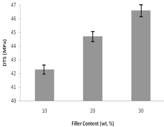
Fig. 7. Diametral tensile strength of the composite samples containing various amounts of nm-size Al<sub>2</sub>O<sub>3</sub> filler particles.
