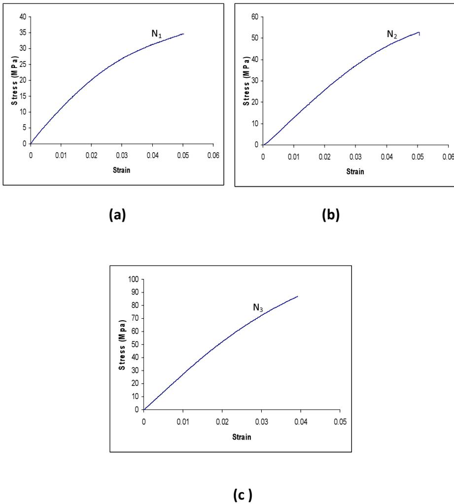
Fig. 6. Stress-strain curves for the composite samples containing various amounts of nm-size Al<sub>2</sub>O<sub>3</sub> filler particles.
