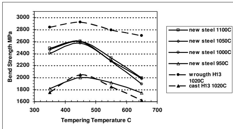
Fig. 6. Bending strength of steels versus tempering temperatures.
