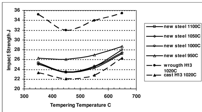
Fig. 8. Impact strength of steels versus tempering temperatures.
