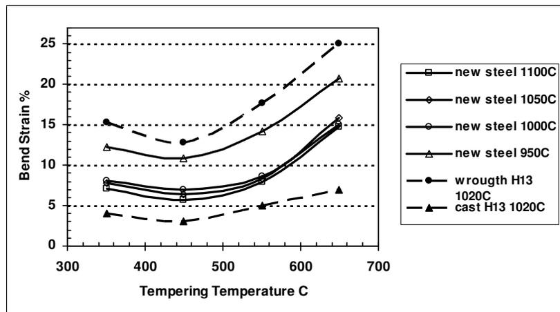
Fig. 7. Bending strain of steels versus tempering temperatures.
