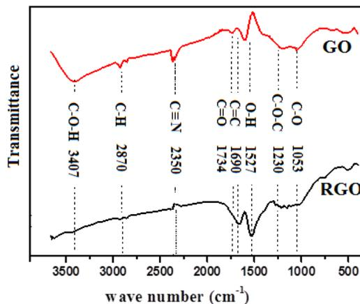
Fig. 8. FTIR spectra for GO and RGO.
