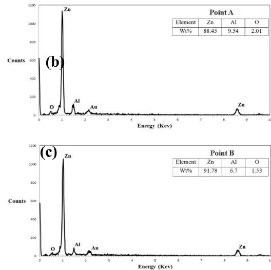
**Fig. 6.** Surface of the oxide film in Zn4Al alloy and respective EDS analysis from the points A and B.
