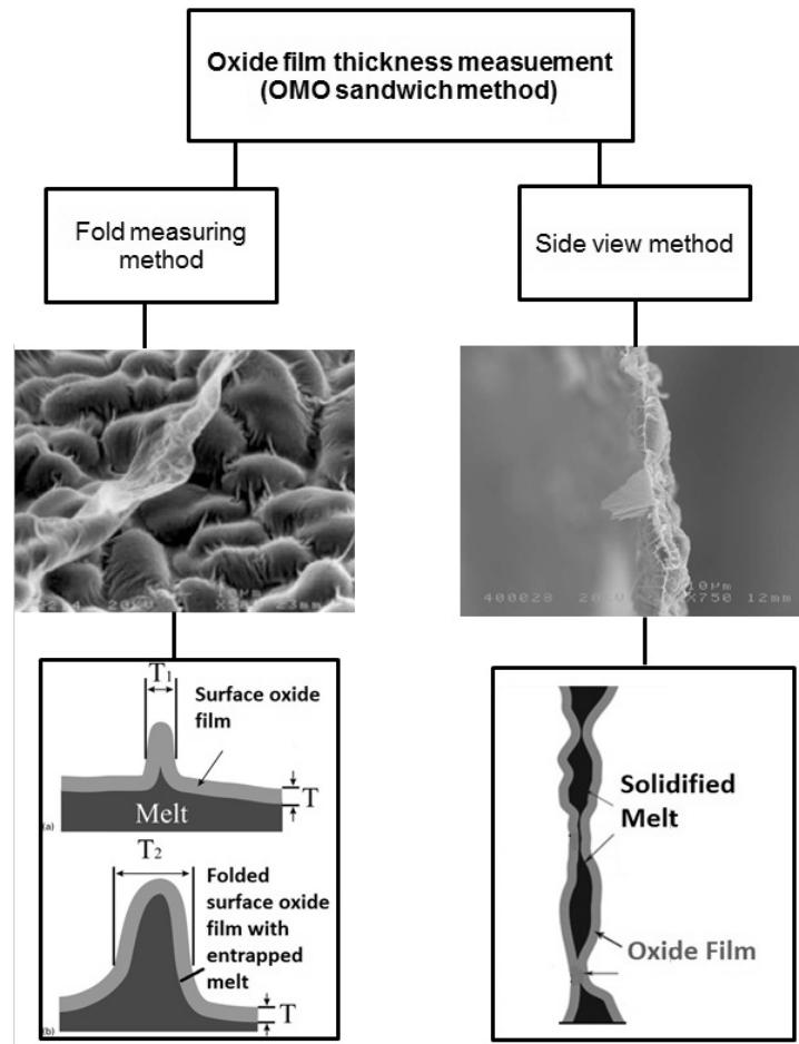
**Fig. 1.** Schematic diagram showing two methods used for measuring oxide film thickness in OMO sandwich .
