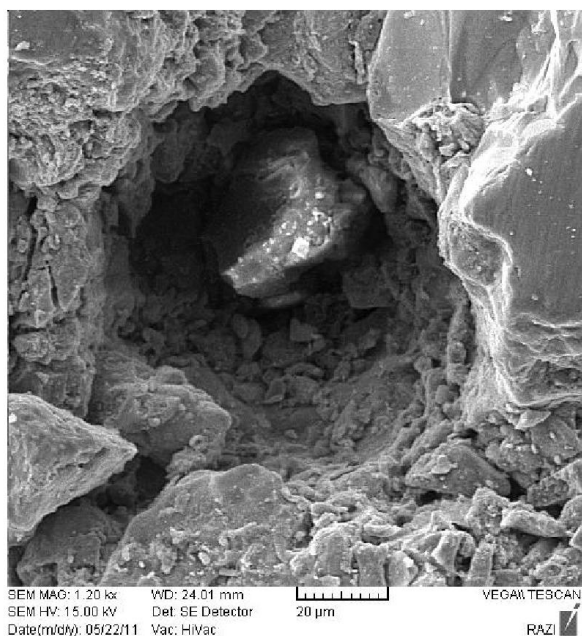
Fig. 5. Pore morphology of porous sample with 10 wt. % bioglass.
