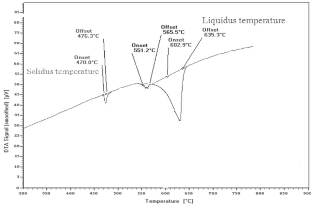
Fig. 6. DTA curveduring heating of the 7075 alloy
