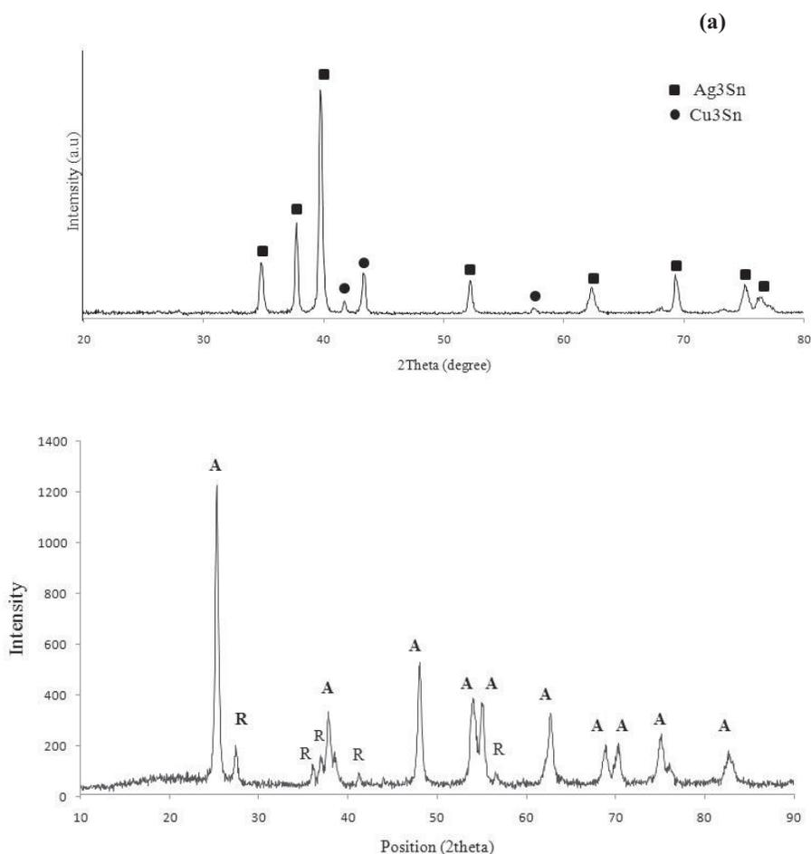
Fig. 1. XRD pattern of a) amalgam alloy powder and b) TiO<sub>2</sub> NPs.
