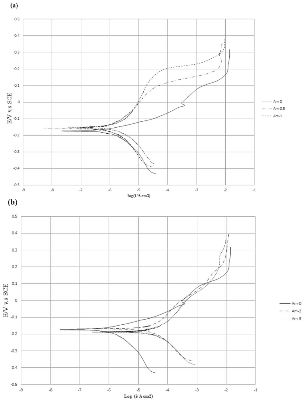
**Fig. 6.** Representative anodic potentiodynamic polarization curves of reference dental amalgam with (a) dental amalgams containing 0.5 and 1 wt% TiO<sub>2</sub> NPs and (b) dental amalgams containing 2 and 3 wt% TiO<sub>2</sub> NPs.
