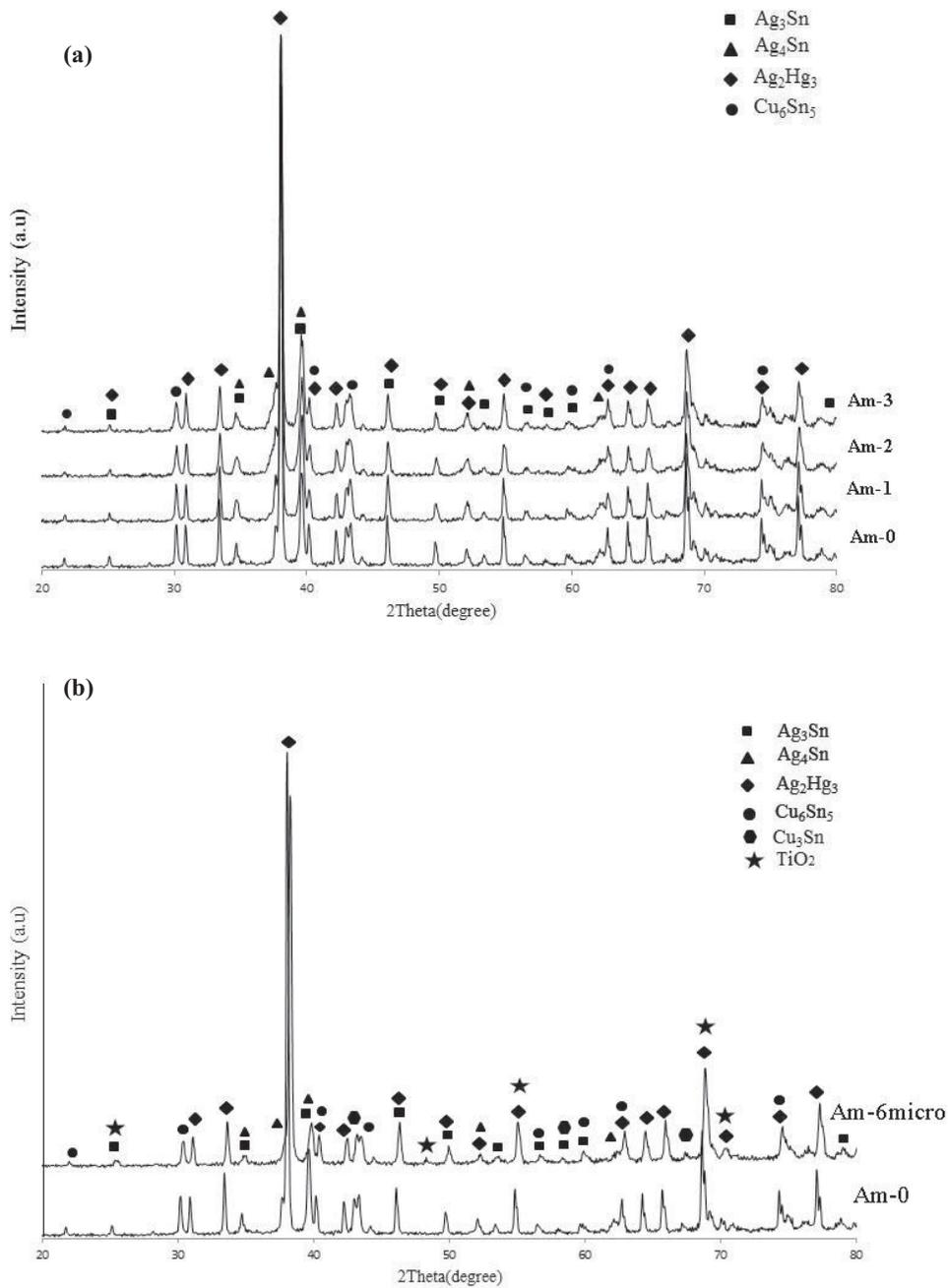
**Fig. 2.** XRD results of reference dental amalgam with (a) dental amalgams containing 1,2and 3 wt% of TiO<sub>2</sub> NPs and (b) dental amalgam with 6wt% micro TiO<sub>2</sub>.
