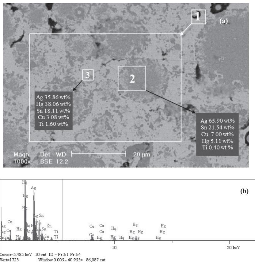
Fig. 5. EDS results of dental amalgam with 1.5 wt% TiO<sub>2</sub> NPs; (a) SEM micrograph and EDS results for 1 and 2 region and (b) spectrum of EDS analysis for the first region.
