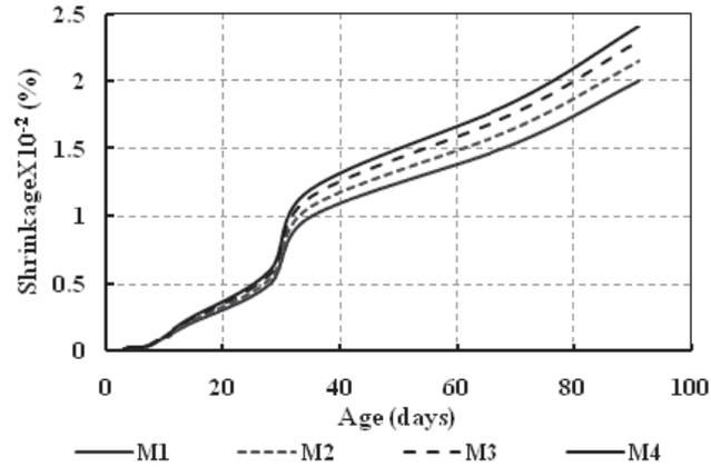
Fig. 5. Dry shrinkage of different mortar mixtures
