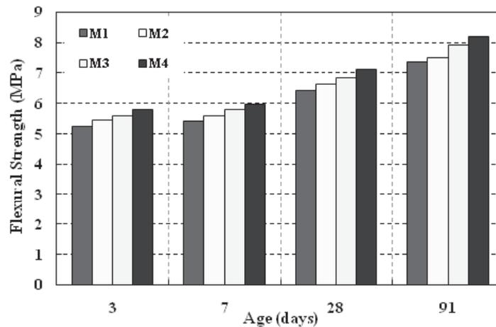
Fig. 4. Flexural strength developments of different concrete mixtures
