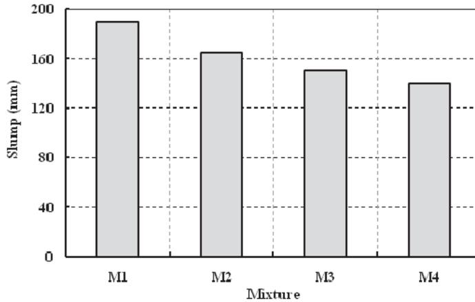
Fig. 1. Initial slump of different concrete mixtures
