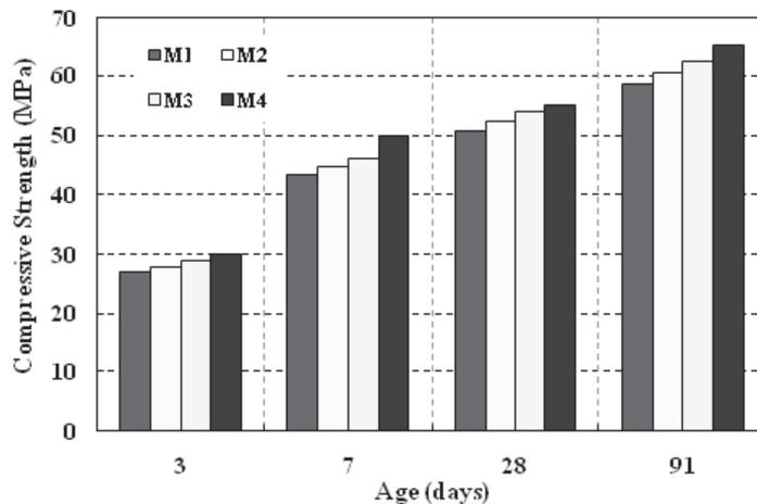
Fig. 2. Compressive strength developments of different concrete mixtures
