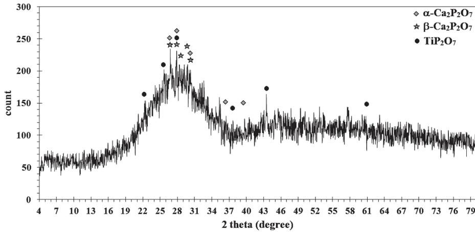
Fig. 3. XRD pattern of CaO-P<sub>2</sub>O<sub>5</sub>-Na<sub>2</sub>O-TiO<sub>2</sub> glass ceramic heat treated at 672 °C for 10 minutes
