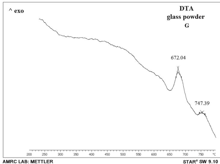
Fig. 2. DTA trace of  $\text{CaO-P}_2\text{O}_5\text{-Na}_2\text{O-TiO}_2$  glass powder
