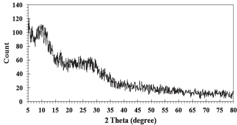
Fig. 1. X ray diffraction of  $\text{CaO-P}_2\text{O}_5\text{-Na}_2\text{O-TiO}_2$  glass powder
