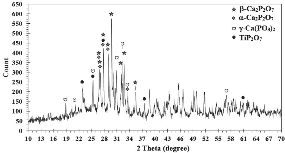
Fig. 4. XRD pattern of CaO-P<sub>2</sub>O<sub>5</sub>-Na<sub>2</sub>O-TiO<sub>2</sub> glass ceramic heat treated at 747 °C for 10 minutes
