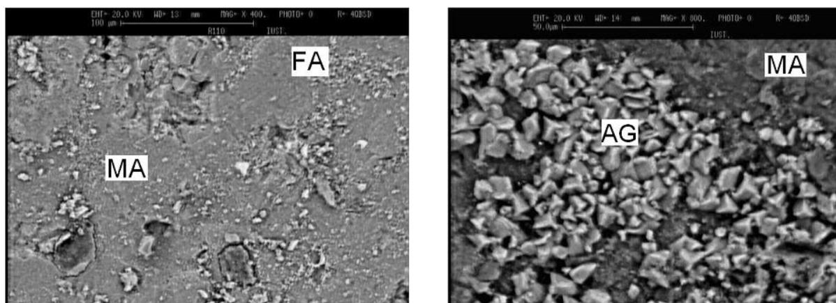
**Fig. 3.** a) Microstructure of sample with optimum content of silica sol after drying showing well dispersed alumina particles (b) with excess amount of silica sol showing the agglomeration of alumina particles.
