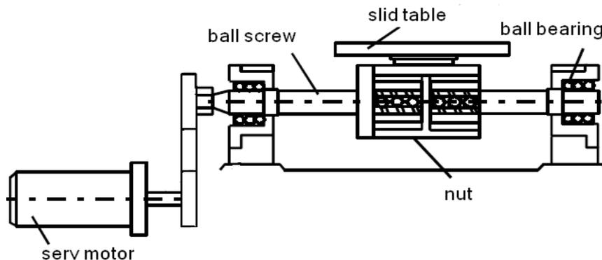
**Fig. 12.** Machine tool feed drive system [15]
