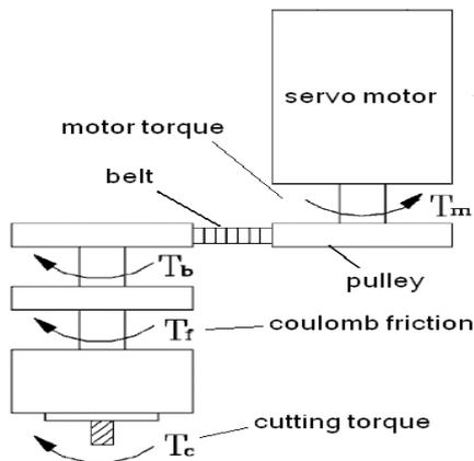
Fig.14. Spindle drive system of the drilling machine [3]
