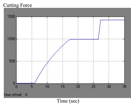
Fig. 7. Simulated cutting force diagram for a new drill: diameter 15.9 mm, point angle 118°, helix angle 33°, pilot hole diameter 3.2 mm, speed 200 rpm, federate 0.102 mm/rev
