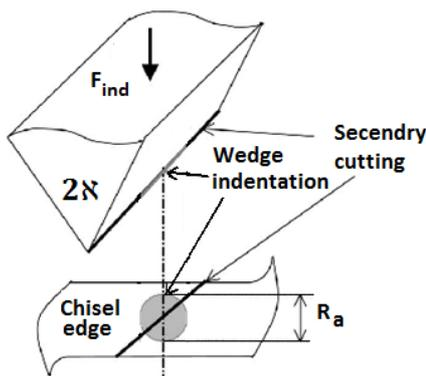
Fig. 4. Chisel edge of the drill [10]
