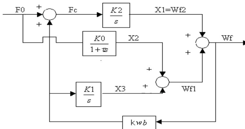
Fig. 9. Block diagram of the wear model [11]
