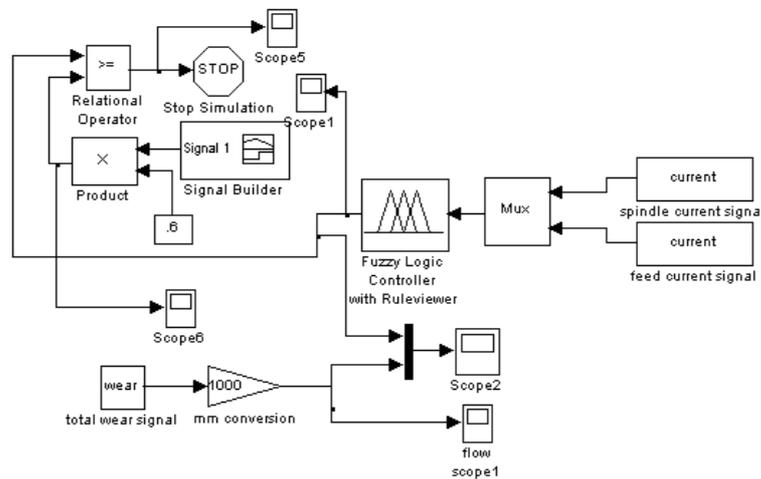
Fig. 24. Simulated model of the fuzzy logic system
