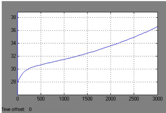
Fig. 17. Simulated feed motor current diagram during drilling: diameter 15.9 mm, point angle 118°, helix angle 33°, pilot hole diameter 3.2 mm, speed 200 rpm, federate 0.102 mm/rev
