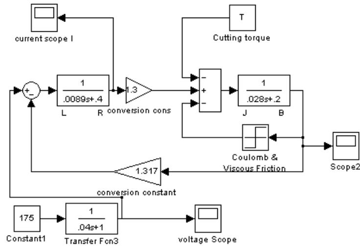
Fig. 16. Simulated block diagram of spindle drive for IHU3 type of motor
