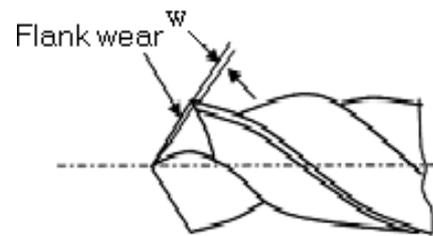
Fig.1. Schematic of a conical point drill [3]
