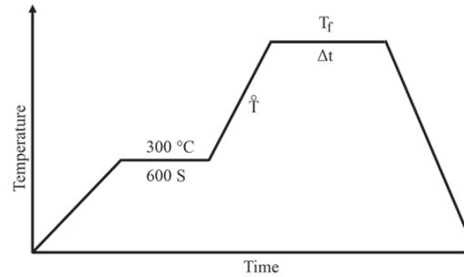
Fig. 3. Heat treating profile used for foaming procedure
