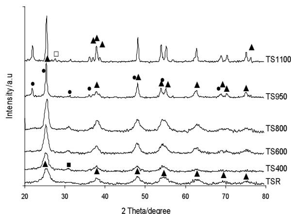
Fig. 2. XRD spectra of as-prepared  $\text{TiO}_2/\text{SiO}_2$  composite and samples heat-treated at different temperatures. ( $\blacktriangle$ ) peaks due to anatase, ( $\square$ ) peaks due to rutile, ( $\blacksquare$ ) peaks due to brookite, and ( $\bullet$ ) peaks due to  $\text{SiO}_2$  (cristobalite).
