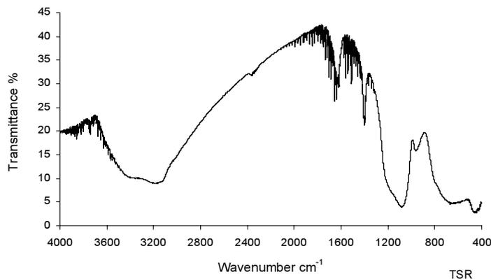
Fig. 1. FTIR spectrum of as-prepared  $\text{TiO}_2/\text{SiO}_2$  composite.
