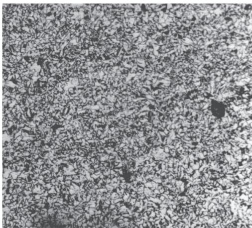
Fig. 6. Microscopic structure of stack plate 2% Nital (x 33)
