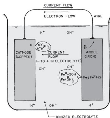
Fig. 1. Schematic diagram of a iron/copper corrosion cell
