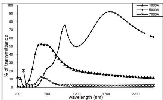
Fig. 5. Variation of transmittance spectra with wavelength for Cu<sub>2</sub>S films of different thicknesses
