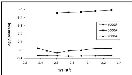
Fig. 4. Variation of resistivity with inverse of temperature for Cu<sub>2</sub>S films of different thicknesses measured at constant current
