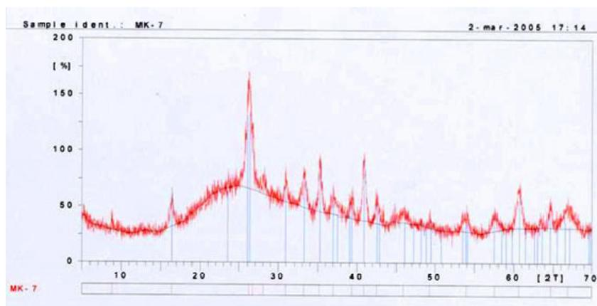
Fig. 4. XRD pattern of the mordenite zeolite membrane
