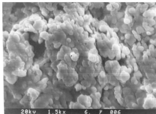
**Fig. 5.** SEM of the mullite support
