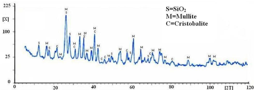
Fig. 3. XRD pattern of the mullite support
