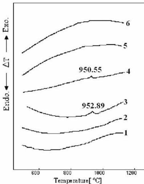
Fig. 1. DTA curves of the glasses S<sub>1</sub>(1), S<sub>2</sub>(2), S<sub>3</sub>(3), S<sub>4</sub>(4), S<sub>5</sub>(5) and S<sub>6</sub>(6)
