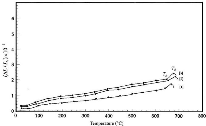
**Fig. 5.** Thermal expansion of ST<sub>3</sub>Z<sub>1</sub> (1), ST<sub>3</sub>Z<sub>1</sub>Y<sub>1</sub> (2) and ST<sub>3</sub>Z<sub>1</sub>C<sub>3</sub> (3) glass ceramics
