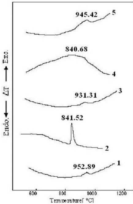
**Fig . 2.** DTA curves of the glasses S(1), ST<sub>3</sub> (2), SZ<sub>4</sub> (3), SP<sub>1</sub> (4) and SY<sub>1</sub> (5)
