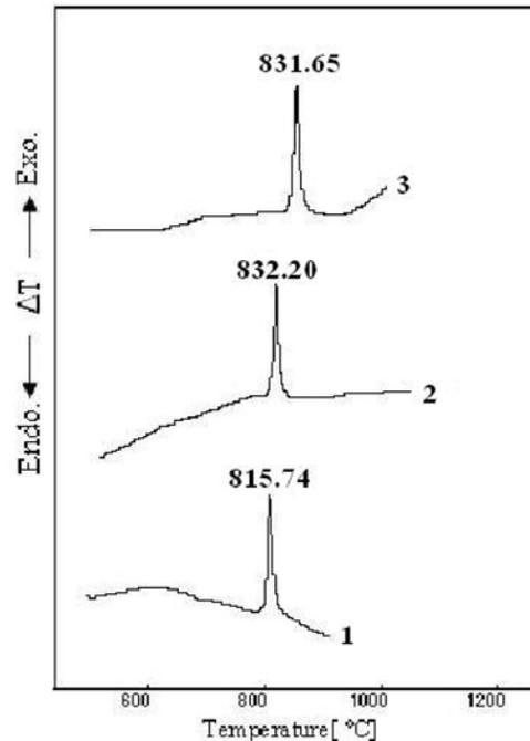
**Fig. 3.** DTA curves of the glasses ST<sub>3</sub>Z<sub>1</sub> (1), ST<sub>3</sub>Z<sub>1</sub>Y<sub>1</sub> (2) and ST<sub>3</sub>Z<sub>1</sub>C<sub>3</sub>(3)
