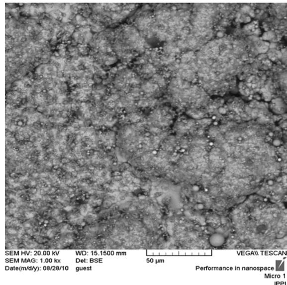
Fig. 3. surface morphology of NiP- $\text{MoS}_2$ - $\text{Cr}_2\text{O}_3$
