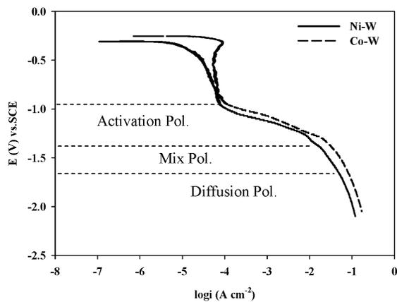
Fig. 1. Cathodic polarization plots of Ni-W and Co-W depositions obtained at room temperature (scan rate = 40 mV s<sup>-1</sup>)
