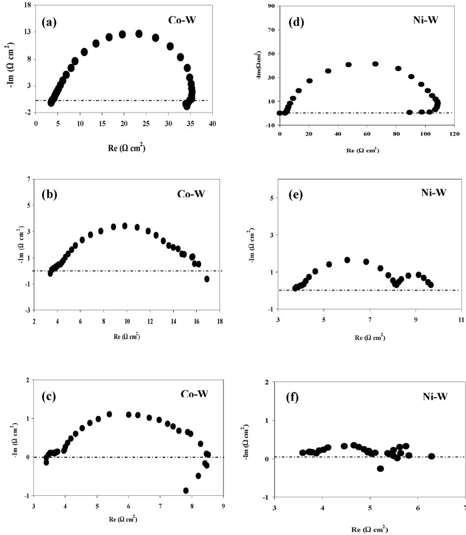
Fig. 4. Nyquist plots of the coatings at: (a, d) 2.5 mA cm<sup>-2</sup>, (b, e) 15 mA cm<sup>-2</sup>, (c, f) 50 mA cm<sup>-2</sup>
