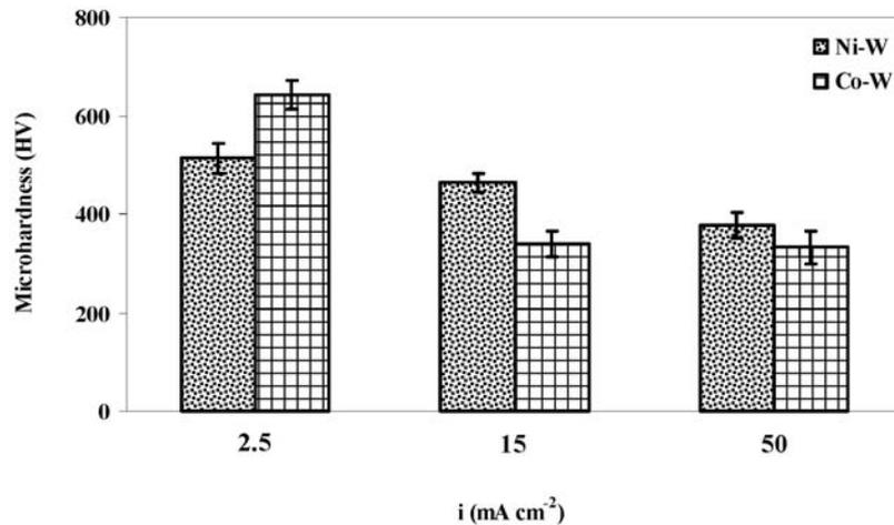
Fig. 7. Microhardness values for Ni-W and Co-W coatings.
