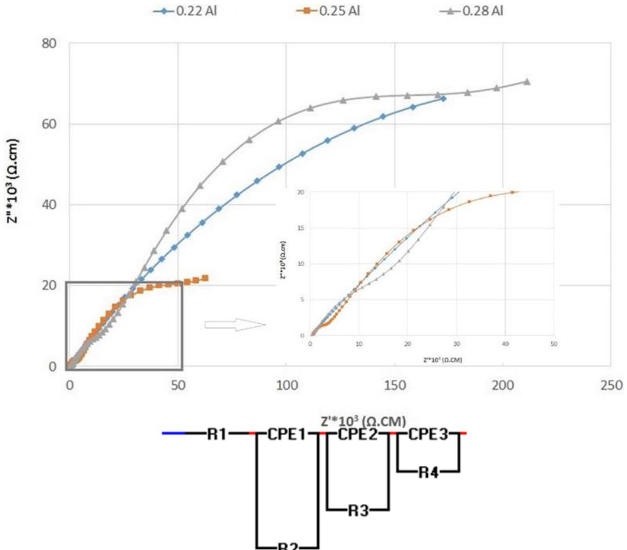
**Fig. 5.** Impedance image of  $\text{Li}_{7-3x}\text{Al}_x\text{La}_3\text{Zr}_2\text{O}_{12}$  garnet ( $x = 0, 0.22, 0.25, \text{ and } 0.28$ ).
