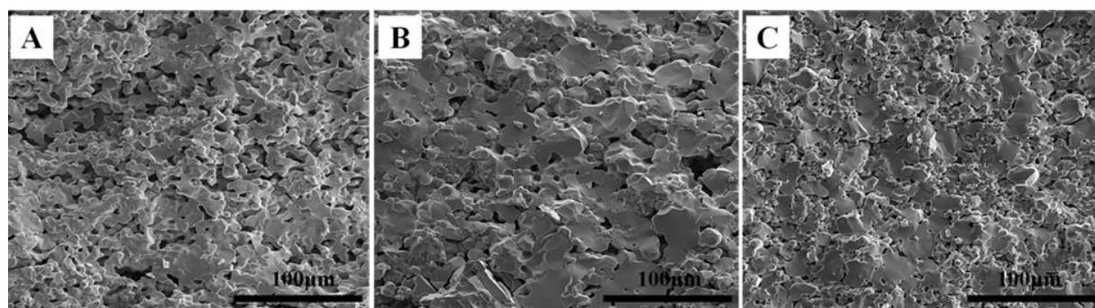
**Fig. 4.** Field emission scanning electron microscope image of the fracture section, a) 0.22 mole of Al additive b) 0.25 mole of Al additive and c) 0.28 mole of Al additive, sintered at  $1180^\circ\text{C}$  for 10 hours.
