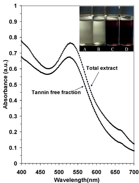
**Fig. 1.** UV-visible spectra of gold colloids: Spectra recorded after adding the ethanol extract of black tea and its tannin free fractions (10ml) to 90 ml of a chloroauric acid solution (1 mM). The curves are recorded after a period of 15 min. The inset shows a photograph of the solutions of chloroauric acid (1 mM) before (A, B) and after exposure to the ethanol extract of black tea (C) and its tannin fraction (D)
