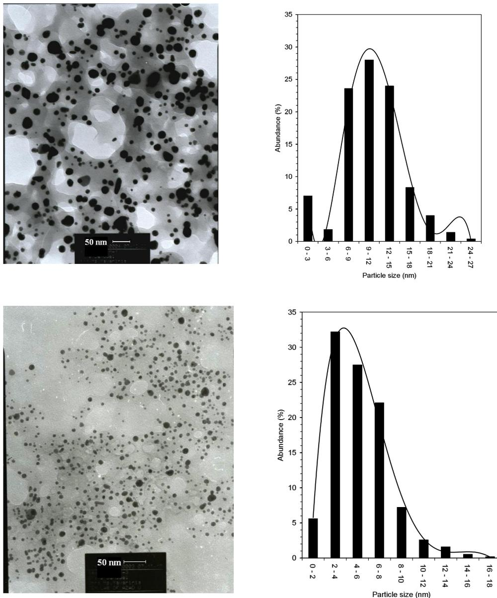
**Fig. 2.** Transmission electron micrographs recorded from a small region of a drop-coated film of chloroauric acid solution treated with the ethanol extract of black tea (upper left picture) and its tannin fraction (lower left picture) for 15 min (scale bars correspond to 50 nm). The related particle size distribution histograms (right side pictures) obtained after counting 350 individual particles for each sample.
