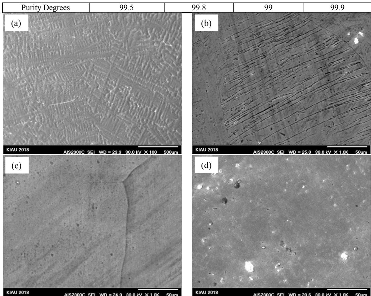
**Fig. 1.** Optical microstructures of the (a) As cast, (b) Hot Forged, (c) Solution Treated and (d) Cold Rolled alloys.
