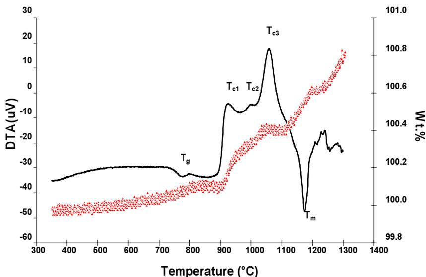
Fig. 6. DTA/TGA plot of glass 28Ca:57Si:15Al:75O:20N:5F eq.%.
