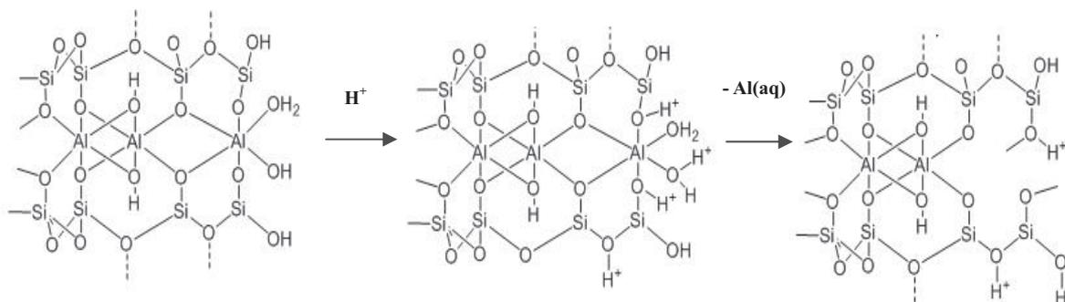
Fig. 1. Schematic of acid activation of montmorillonite
