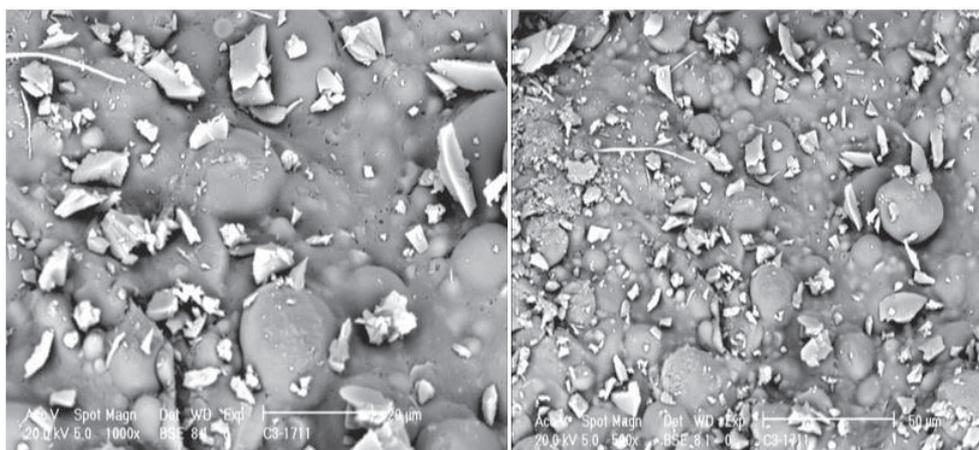
Fig. 3. SEM images of  $TiO_2$ -pillared montmorillonite
