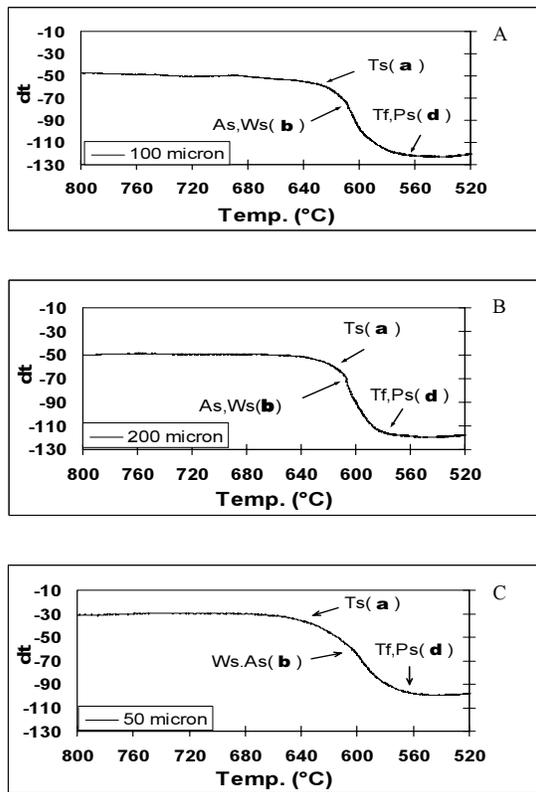
**Fig. 4.** Illustration of grain boundary ferrite and intragranular start temperatures and end of reaction for:
