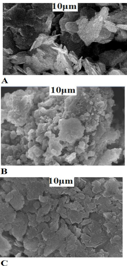
**Fig. 2.** SEM pictures of clay samples. A KAO: B KAO-H<sub>2</sub>SO<sub>4</sub>: C KAO-NaOH
