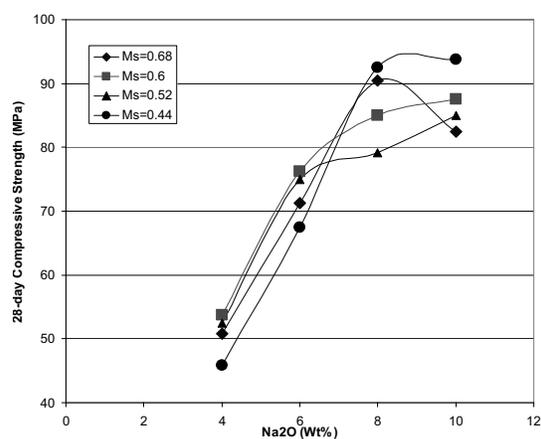
**Fig. 3.** Effects of Na<sub>2</sub>O concentration on compressive strength development at hydrothermal curing condition.
