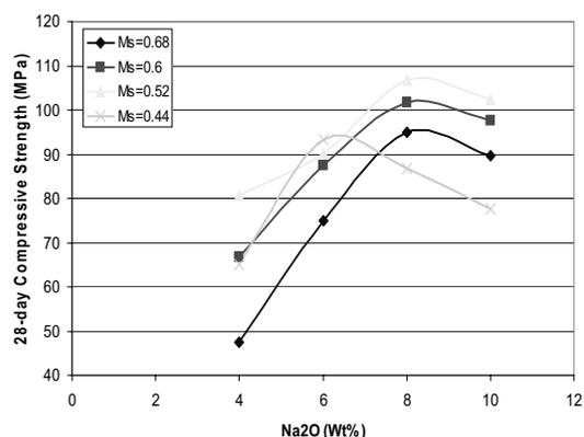
**Fig. 2.** Effects of Na<sub>2</sub>O concentration on 28-day compressive strength development at 95% R.H. at 25°.
