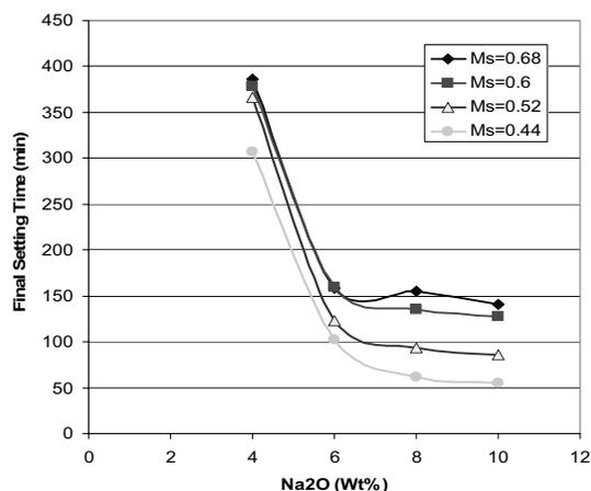
**Fig. 1.** Effect of Na<sub>2</sub>O concentration on final setting time.
