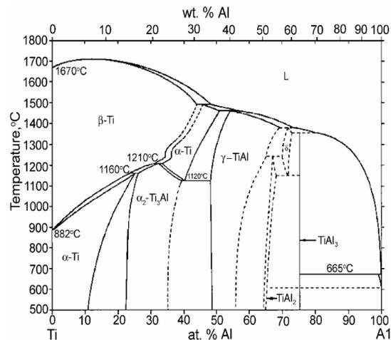
Fig. 1. Ti-Al phase diagram [8].
