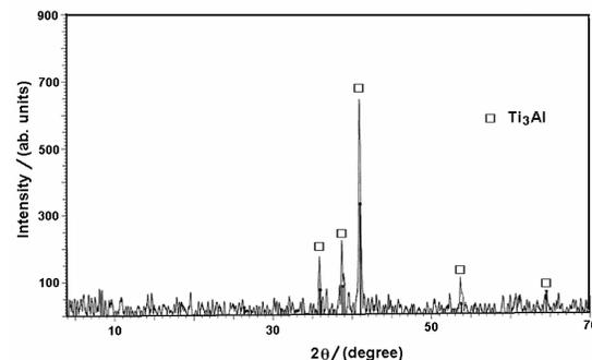
Fig. 10. XRD analysis from granulate 3 of Fig. 7.
