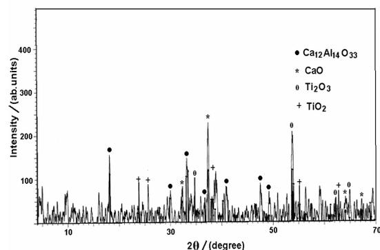
Fig. 8. XRD analysis from granulate 1 of Fig. 7.
