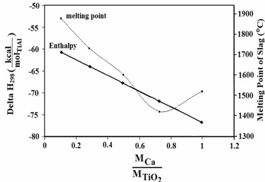
**Fig. 6.** Enthalpy of different reactions in TiO<sub>2</sub>-Al-Ca system for production of 1 mole of TiAl as well as melting point of calcoaluminat slags versus M<sub>Ca</sub>/M<sub>TiO<sub>2</sub></sub> (M: mole).
