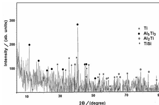
Fig. 11. XRD analysis from granulate 4 of Fig. 7.
