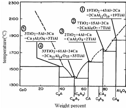
**Fig. 5.** Situation of different calcoaluminate products in CaO-Al<sub>2</sub>O<sub>3</sub> phase diagram.
