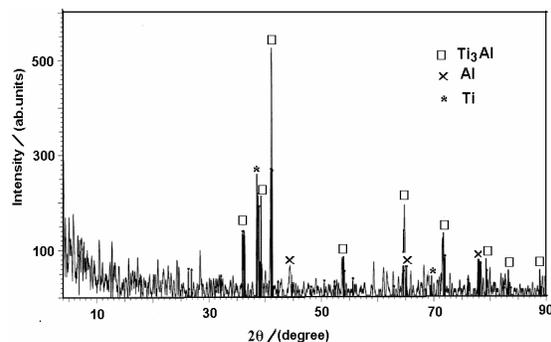
Fig. 9. XRD analysis from granulate 2 of Fig. 7.
