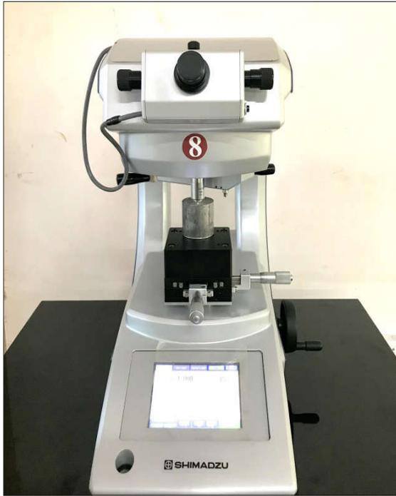
Fig. 2. Specimen loaded on (Shimadzu) hardness tester
