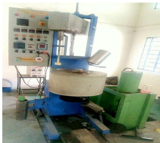
**Fig. 1.** Squeeze casting machine setup
