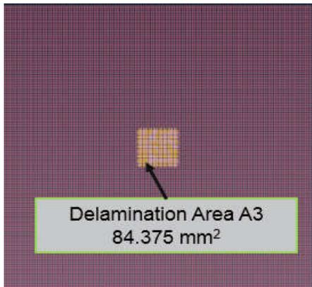
Fig. 3. Top view of delamination incorporated.
