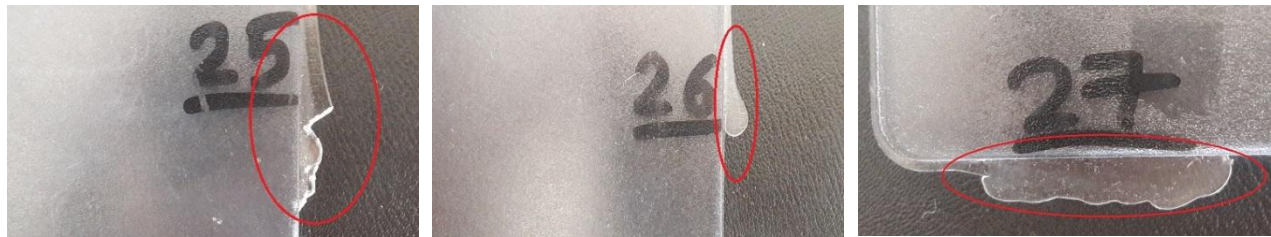
Fig. 9: The plated PC samples with holding pressure time of 2.5 s and cooling time of 20 s
